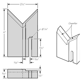
Figure 5: Outfeed support V-block (adjustable).
