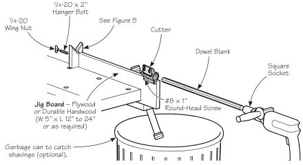
Figure 3: Alternative dowel-making set-up.
