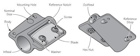
Figure 1: Dowel and tenon cutter components.
